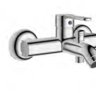
EXPOSED BATH MIXER WITH SHOWER KIT 40mm Ceramic Cartridge, Single Body, Brass Cast, Wall Spout Length 140mm, Hand Shower, Wall Bracket, Shower Hose
