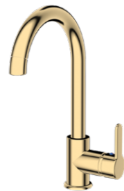
SINGLE-LEVER SINK MIXER WITH MOVABLE SPOUT 35 mm Ceramic Cartridge, 50 cm 1st Quality Flex Connection, Single Screw Easy Installation, Pipe End Water Flow Height 190mm, Outlet End Length 125mm
